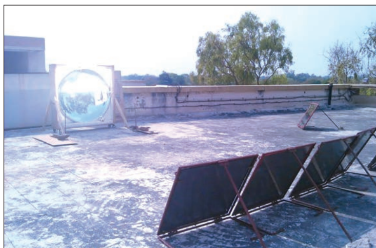
The arrangement of flat reflecting surfaces reflecting sunlight on a large concave mirror.
