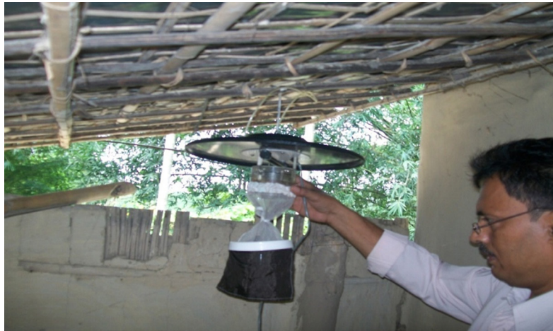
Figure 2. Application of battery-operated CDC miniature light trap for sampling mosquito adult populations in human dwellings can help ascertain mosquito fauna and supplement mosquito collections in the given locality.
